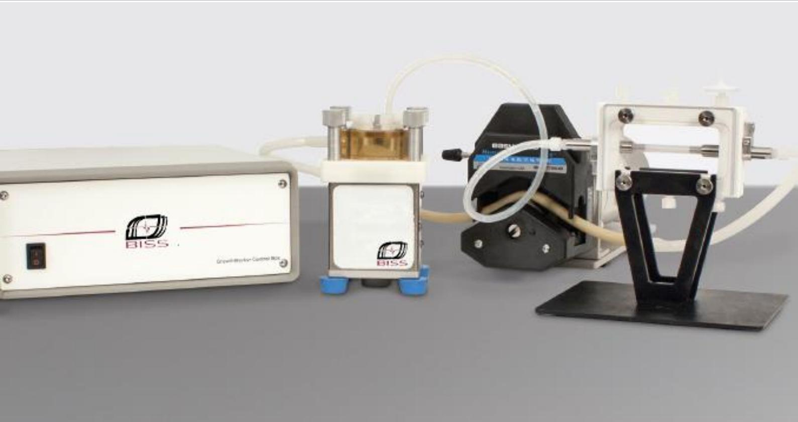
BiSS bioreactors provide a controllable, 3D environment for stimulating physiological conditions in vitro. The LumeGen imparts mechanical pulsatile pressure to a 3D sample. Applications include investigating cell function, modulating the growth and development of engineered tissues, or acting as a test bed for drug and regenerative medicine technologies.
