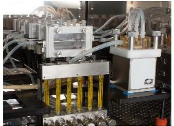
LumeGen Bioreactor System with Six Chambers
